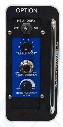
The controls for the DSP3 Helium Speech Unscrambler (HSU) are located in the options panel on the right side of the front panel as shown below.
