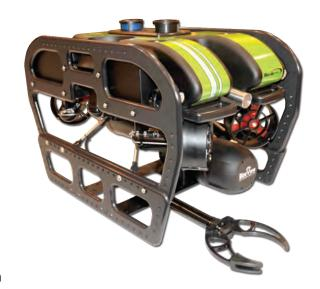
The vLBV950 operates at depths to 950 meters (over 3,000 ft), using our advanced 100mm propellers for leading edge performance in its class. Various deployment configurations are available from free-swimming, to TMS (tether management systems), to LARS (launch and recovery systems).
